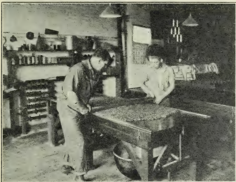
FIG. 32.—Rolling out peanut candy, preparatory to cutting it up into 5-cent bars. The iron "rails" at the sides of the table keep the candy to a uniform thickness
